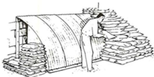
A Four-person Basement Shelter Made of Curved Asbestos-Cement Sheets Covered With Sandbags.
