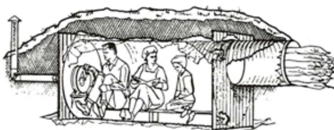
A Backyard Corrugated Steel Pipe Shelter.
