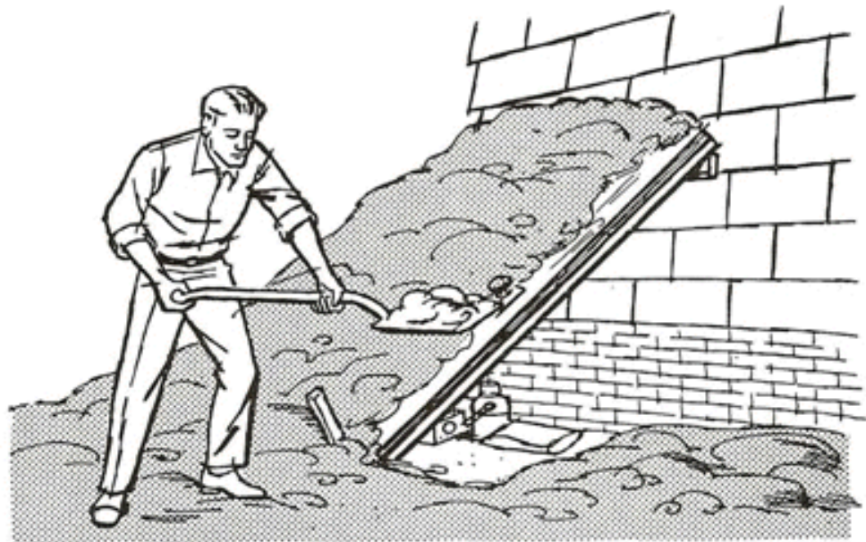
FIGURE 57.—Improvising backyard covered shelter.
